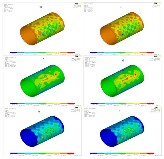
Fig. 9. Pile construction is completed stage 1 Lining Y direction displacement contours (a), pile construction completed Phase 2 Lining Y-direction displacement (b), pile construction is completed stage 1 Lining X-direction displacement contours (c), pile Phase 2 construction is completed lining X-direction displacement contours (d), pile Phase-1 construction is completed lining combined displacement contours (e), pile Phase-2 construction is completed lining combined displacement contours (f)
