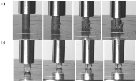
Fig. 2. Crushing test schemes: a - vertical crushing; b - horizontal crushing
