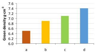
Fig. 6. Change in the pressing density depending on the specific energy of discharge 0.8; 0.9; 1.0 and 1.2 kJ·cm<sup>-3</sup>
