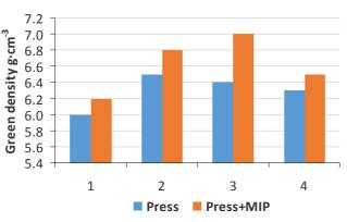
Fig. 5. Change in the density of different powder compositions under static and static-dynamic compaction
