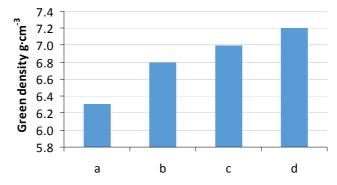
Fig. 7. Change in the pressing density depending on a number of pulses: a - 0; b - 5; c - 10; d - 15 at the specific energy of discharge 0.9 kJ·cm<sup>-3</sup>
