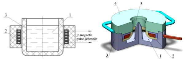
Fig. 2. Technological scheme of pulse-magnetic processing of solutions and suspensions: 1 – material; 2 – inductor; 3 – heating device; 4 – mold; 5 – location of the cover
