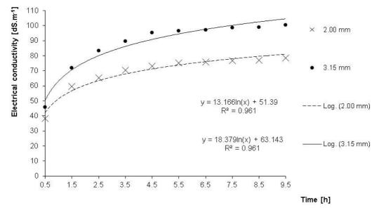
Fig. 4. Graph of time dependence on electrical conductivity for the two significant sieve sizes
