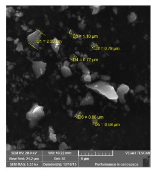
Fig. 3. Detail of the grain fraction *x*<20 micron of sample 1
