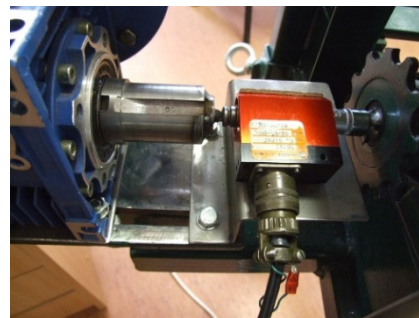
Fig. 3. Torque sensor mounted on the equipment
