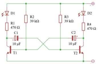
Fig. 1. Scheme of multivibrator
