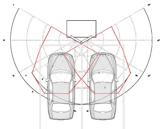
Fig. 5. RFID antennas turned by 30°, cars parked frontward
