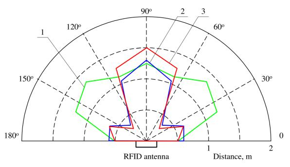
Fig. 3. **RFID** antenna and transponder safe communication field, angle 45°, **RFID** transponder height above the ground: 1 - 20 cm, 2 - 40 cm, 3 - 60 cm
