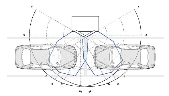
Fig. 6. **RFID antennas turned by 30°, cars parked sideward**
