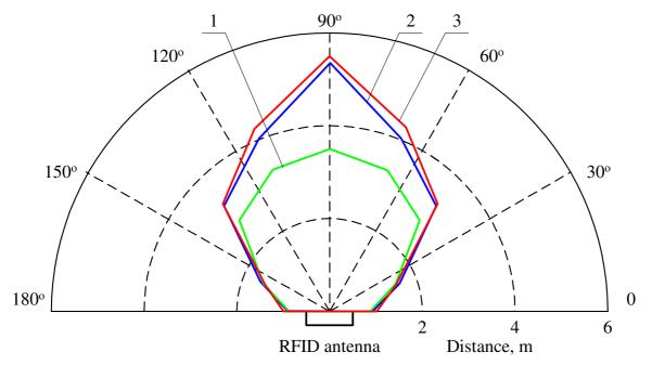
Fig. 2. **RFID antenna and transponder safe communication field, angle 90°:** RFID transponder height above the ground: 1- 20cm, 2- 40cm, 3- 60cm.
