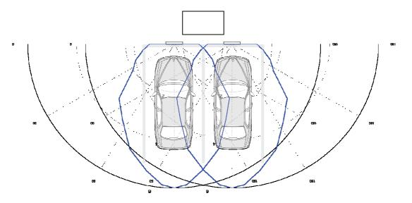
Fig. 4. Electric cars positioned in front of charging station (transponder in the licence plate is parallel to the antenna plane)
