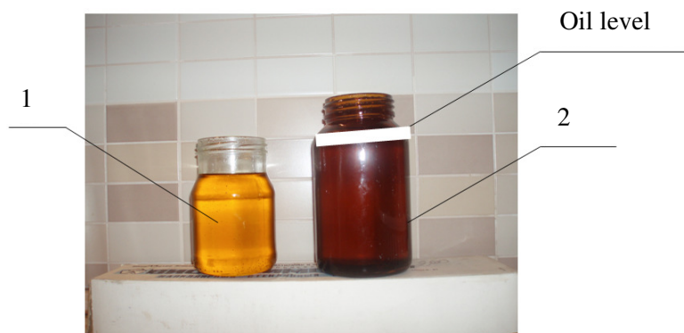
Fig. 1. Fractionation product volume: 1 – 310 ml of separated fraction; 2 – 500 ml of oil
