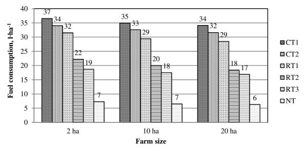
Fig. 3. Fuel consumption of different tillage and sowing systems for different farm size
