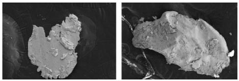
Fig. 1. Shape of fatigue particle [2]
