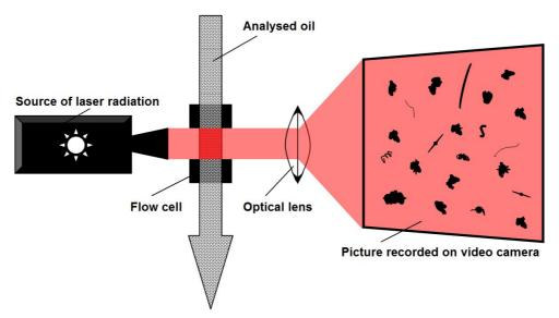
Fig. 2. Principle of LNF analysis [6]
