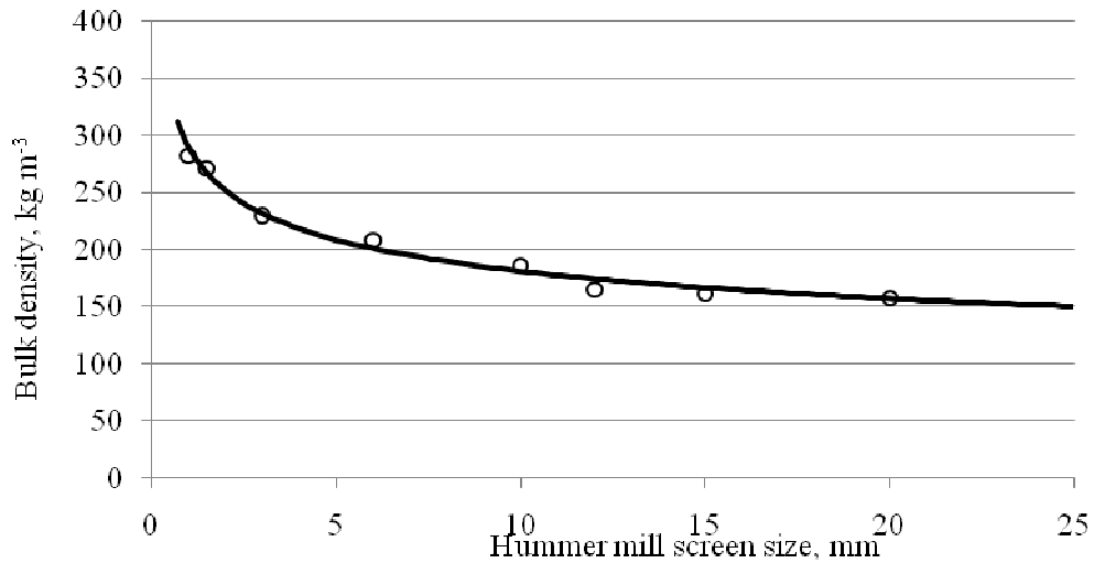
Fig. 2. Bulk density dependence on hammer mill screen size
