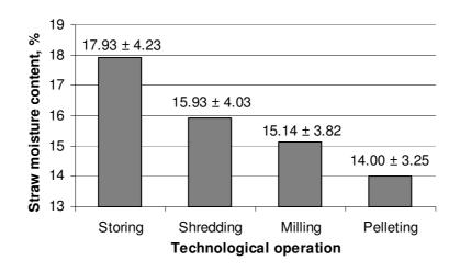
Fig. 2. Variations of straw moisture content in the technological line
