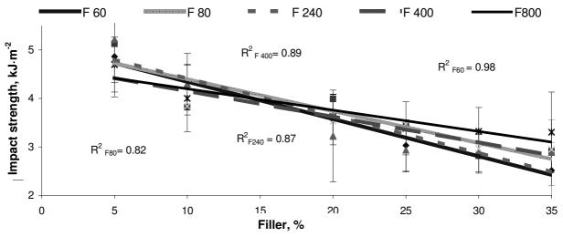
Fig. 2. Influence of filler share in matrix on impact strength of polymeric particle composites with waste-corundum-based filler
