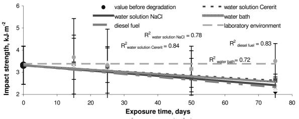
Fig. 3. Influence of degradation on impact strength
