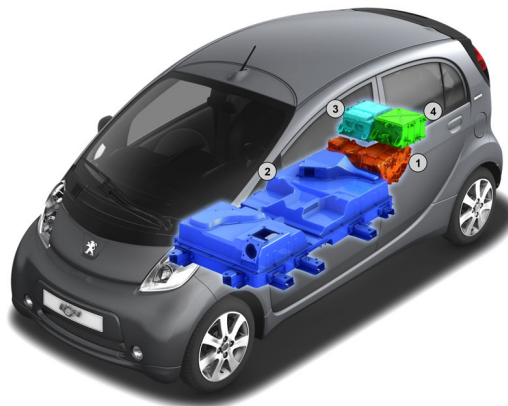
Fig. 4. Battery compartment location in Mitsubishi i-MiEV : 1 – motor; 2 – lithium-ion battery compartment; 3 – inverter; 4 – charger
