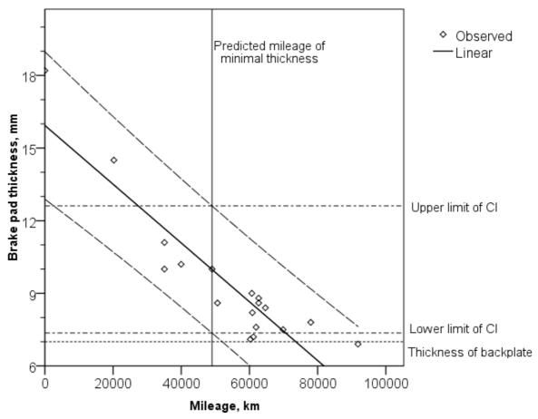
Fig. 4. Results of prediction, Renault Master III, front inner pad
