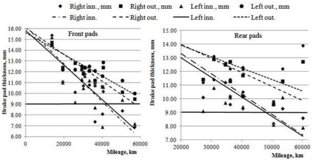
Fig. 1. Brake pad wear data, Renault Trafic II
