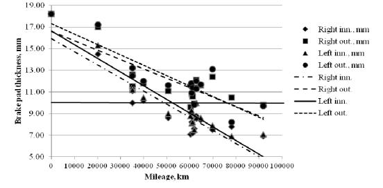
Fig. 2. Brake pad wear data, Renault Master III, front pads
