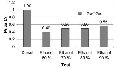
Fig. 3. Formation of limit price of bioethanol with different ethanol content depending on the cost price of diesel fuel
