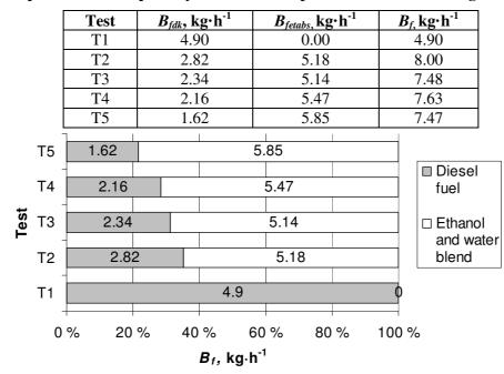
Comparisons of the quantity of fuel consumption in the course of engine testing
