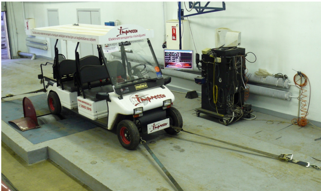
Fig. 2. Slow-moving electric motor vehicle Melex 963DS on power stand.
