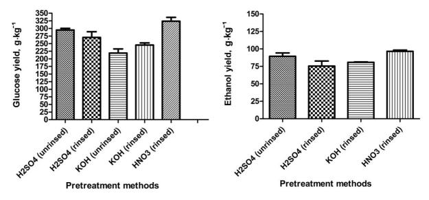
Fig. 1. Influence of different pretreatment methods on glucose yield from rye straw samples
