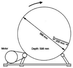
Fig. 1 Briquette durability tester
