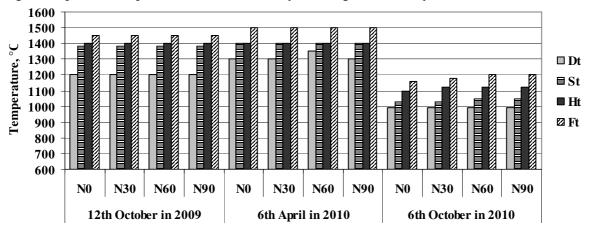
Fig. 1. Ash melting behaviour oxidizing atmosphere depending on the reed canary grass variety "Marathon" harvesting time, and N fertilizer rates: Dt – deformation temperature, St – sphere temperature, Ht – hemisphere temperature, Ft – flow temperature
