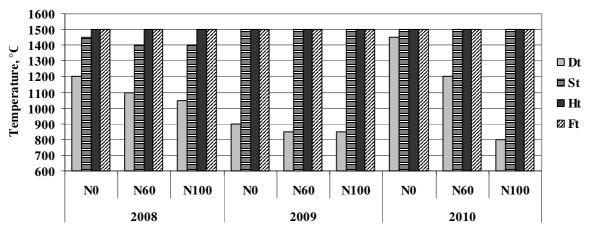
Fig. 2. Ash melting behaviour oxidizing atmosphere depending on the local hemp "Pūriņi" growing year, and N fertilizer rates: Dt – deformation temperature, St – sphere temperature, Ht – hemisphere temperature, Ft – flow temperature
