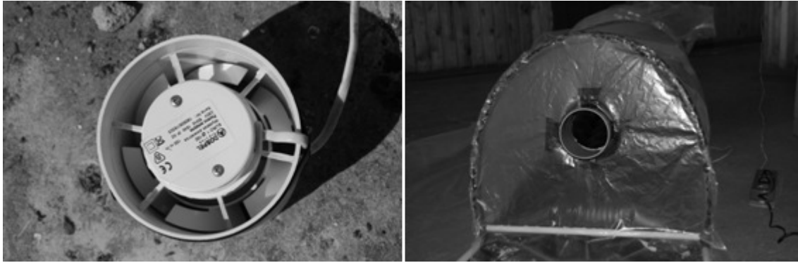
Fig. 2. Fan and its connection port
