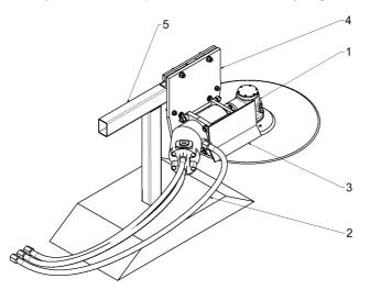
Fig. 3. Laboratory set of mechanical pruner design: 1 – rear transmission with axial piston hydromotor; 2 – hydraulic lines; 3 – little plough blade; 4 – clamping plate; 5 – frame for laboratory measurement
