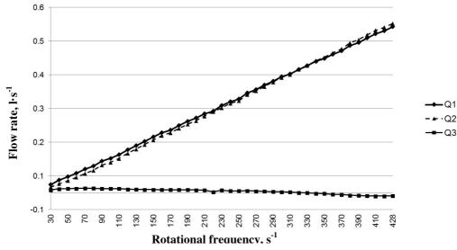
Fig. 5. Graph of dependancy of hydraulic oil flow on cutting disc rotational frequency: Q1 – hydraulic oil flow in pressure line; Q2 – hydraulic oil flow in drain line; Q3 – calculated flow of leakage fluid
