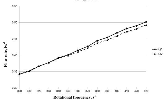
Fig. 6. Details of graph depicting dependency of hydraulic oil flow on cutting disc rotational frequency: Q1 – flow of hydraulic oil in pressure line; Q2 – flow of hydraulic oil in drain line
