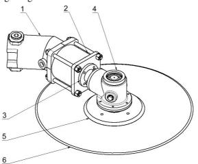
Fig. 2. **Rear transmission with hydromotor:** 1 – axial piston hydromotor; 2 – coupler; 3 – extension; 4 – angular gear; 5 – carrier; 6 – cutting disc
