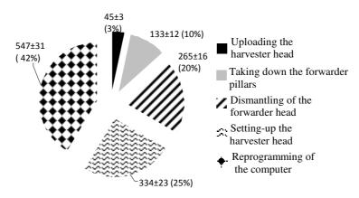
Fig. 1. Stages of the forwarder into harvester transformation (s)
