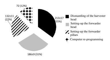
Fig. 2. Stages of the harvester into forwarder transformation (s)
