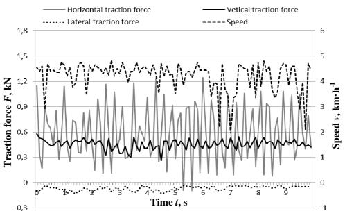
Fig. 2. Traction forces of hob coulter in the soil of 0.044 MPa hardness
