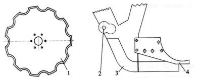
Fig. 1. Complex sowing coulter parts: 1 – disc knife with notched blades; 2 – mounting place of the disc knife; 3 – hob coulter with extended hob; 4 – mount of sowing apparatus
