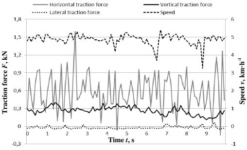
Fig. 3. Traction forces of hob coulter in the soil of 0.493 MPa hardness
