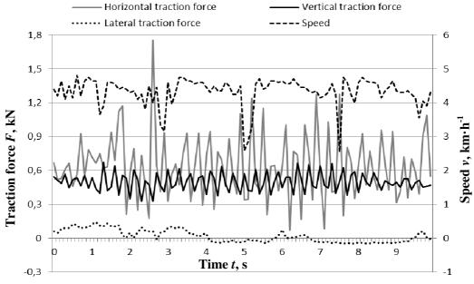
Fig. 5. Traction forces of complex coulter in the soil of 0.044 MPa hardness
