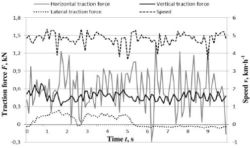
Fig. 7. Traction forces of complex coulter in the soil of 0.827 MPa hardness
