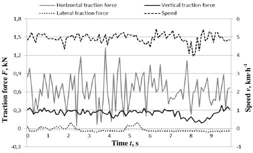
Fig. 6. Traction forces of complex coulter in the soil of 0.493 MPa hardness
