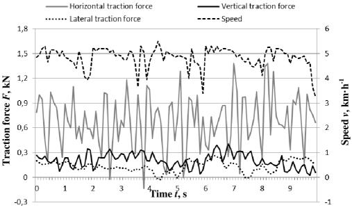
Fig. 4. Traction forces of hob coulter in the soil of 0827 MPa hardness
