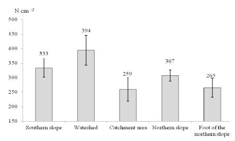
Fig. 8. Soil penetrometric resistance, N·cm<sup>-2</sup>, in soil subsoil layer at depth of 0.2-0.5 m in average per three trial years in trial field No. 2
