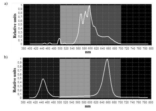
Fig. 1. Ranges of radiation for sodium lamps (a) and LED (b)
