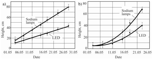
Fig. 2. Growth dynamics of seedlings under sodium lamps and LED for tomatoes (a) and cucumbers (b)
