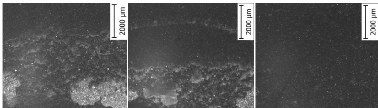
Fig. 3. Adhesive bond failure: (from left: 1:5 15 % SCF, 1:5 30 % SCF, F800 30 % AF)
