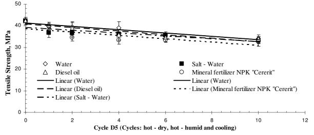
Fig. 2. Effect of environment degradation on tensile strength of adhesive
