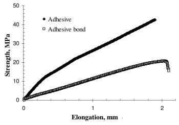
Fig. 3. Tension diagram of adhesive and adhesive bond
