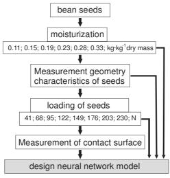
Fig. 1. Diagram of the experiment
