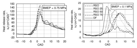
Fig. 3. Amount of RSO in blend influence on heat release rate ( $n = 1400 \text{ min}^{-1}$ )
