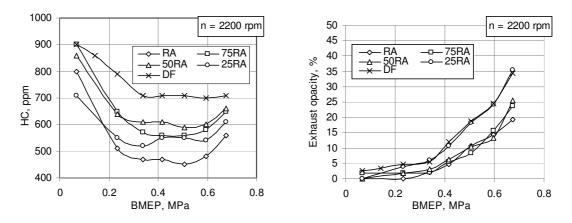
Fig. 6. Influence of the amount of RSO in fuel on HC emissions and exhaust opacity
