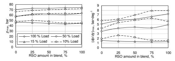
Fig. 2. In-cylinder pressure peak  $(p_{max})$  and maximum cylinder pressure gradient  $((dp/d\varphi)_{max})$  as functions of RSO amount in fuel:  $-n = 1400 \text{ min}^{-1}$ ;  $--n = 2200 \text{ min}^{-1}$
