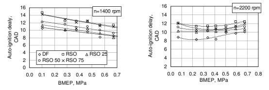
Fig. 1. Dependency of auto-ignition delay on engine load and rapeseed oil amount in the fuel
