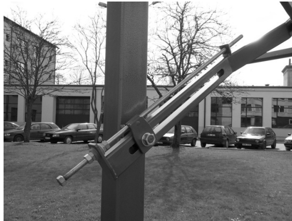
Fig. 6. Angle adjustment mechanism of the solar station
