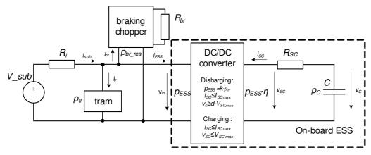
Fig. 1. Block diagram of electric transport feeding system and tram equipped with ESS
