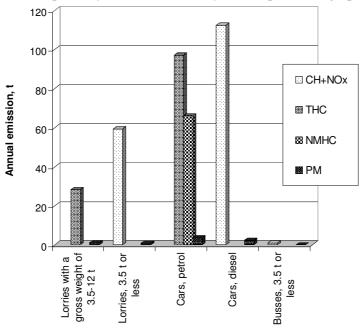
Fig. 2. Annual CH, NO<sub>x</sub> and PM emissions from 10 % of the vehicle fleet of Latvia
