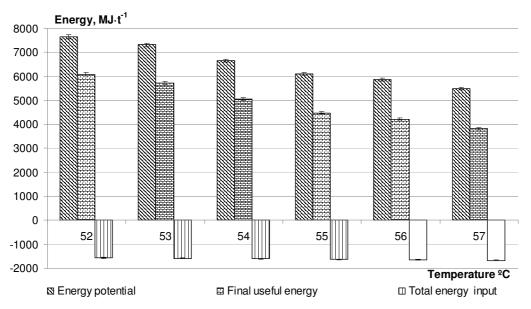
Fig. 3. Energy balances of biogas production using different temperatures
