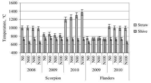
Fig. 2. Ash melting deformation temperature of linseed in Latvia depending on experiment year, variety and N fertiliser norm
