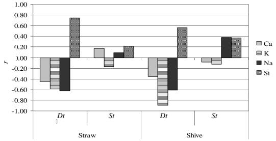
Fig. 1. Hemp (n = 15) correlations between ash melting temperature and chemical content: Dt – deformation temperature; St – sphere temperature
