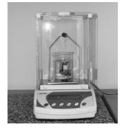
Fig. 4. Stand for determining the specific density
