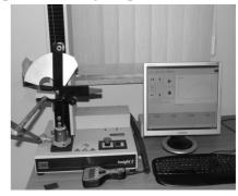
Fig. 2. Stand for determining the static work of cut plant materials: a – cutting device, b – control unit (PC) with software TestWorks 4
