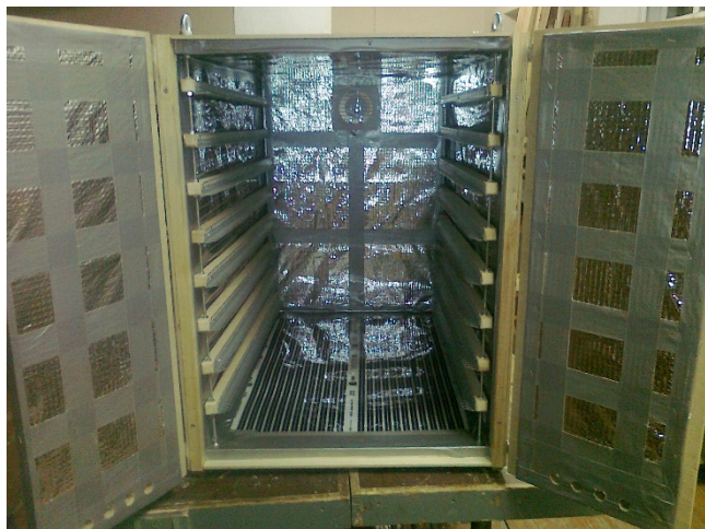
Fig. 2. IR dryer shelving system
