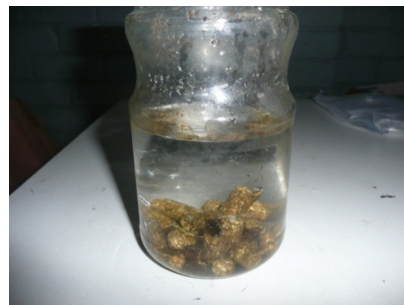
Fig. 2. Hay pellets do not float in liquid
