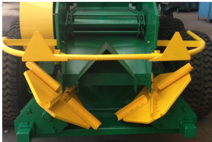
Fig. 7. Mineral spreader with scattering discs, inclined at an angle to the horizon
