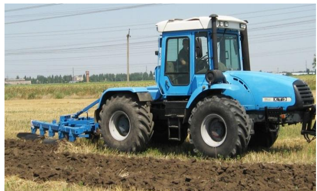
Fig. 6. Arable machine-tractor aggregate based on the HTZ-170 tractor with tires 23.1R26
