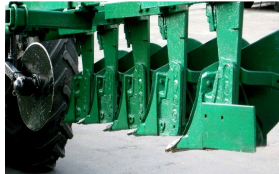
Fig. 4. View of a plough with a field board on its last cowl
