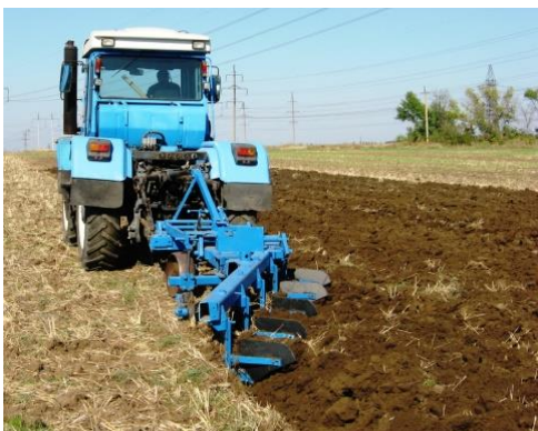
Fig. 5. Arable machine-tractor aggregate based on the HTZ-170 tractor with tires 16.9 \times 38
