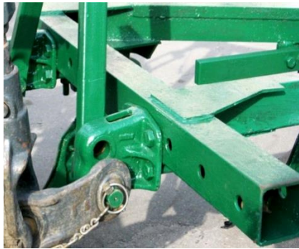
Fig. 3. Placement of the plough attachment bracket on the cowl
