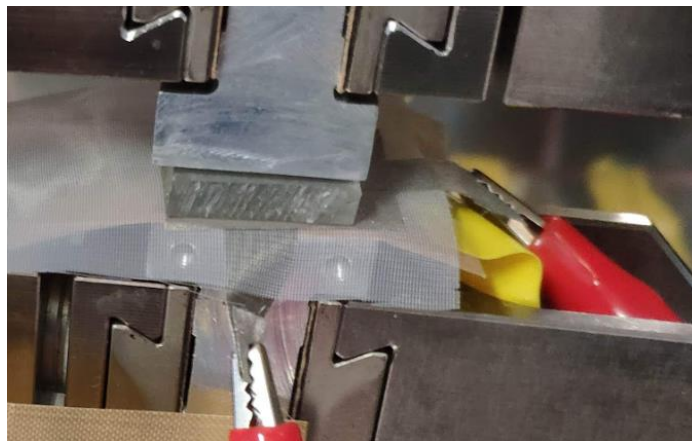
Fig. 2. Connection to Zwick using self-adhesive strips
