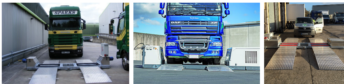
1. att. Ruļļu bremžu stendi “ BM Test Equipment BM20200 ”, “ Hartex engineering MBT 5251 ” un “ Sherpa BPS Mobile ”
