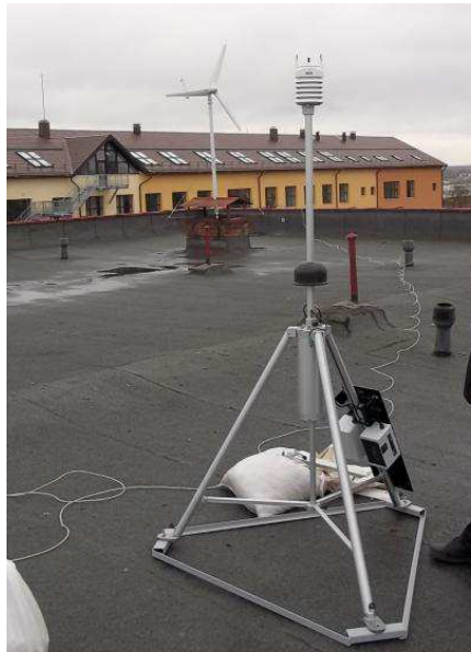
Fig. 3. Vaisala weather station MAWS201 and 300 W wind generator
