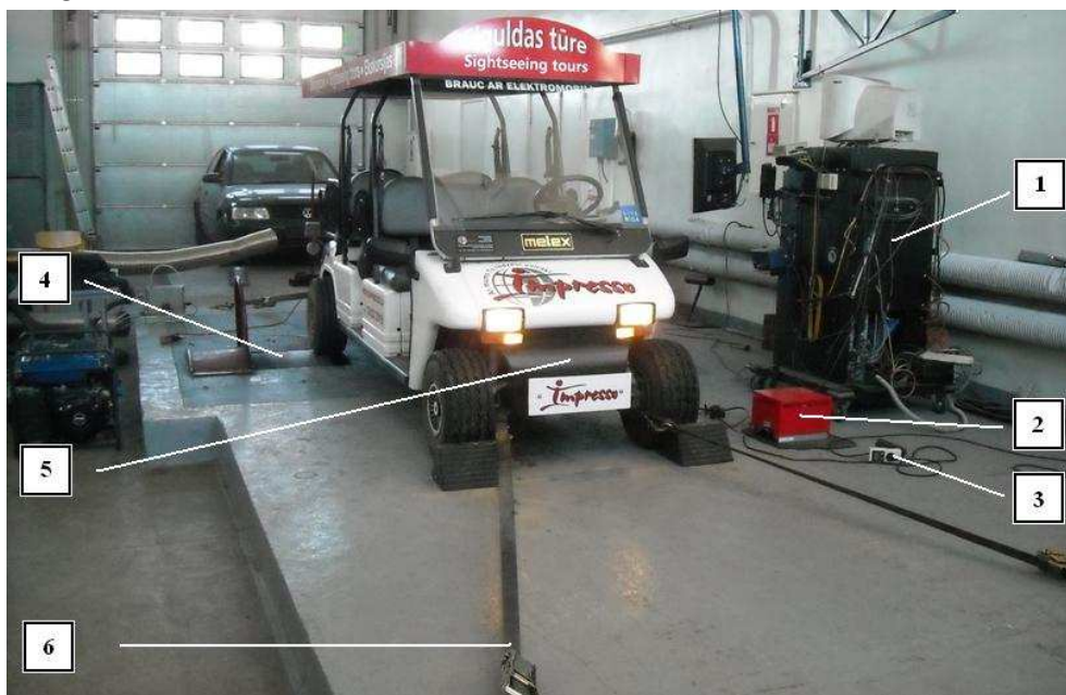
Fig. 1. Melex 963DS on a chassis dynamometer: 1 – control platform, 2 – charger, 3 – REV logger, 4 – chassis dynamometer rolls, 5 – experiment object, 6 – straps
