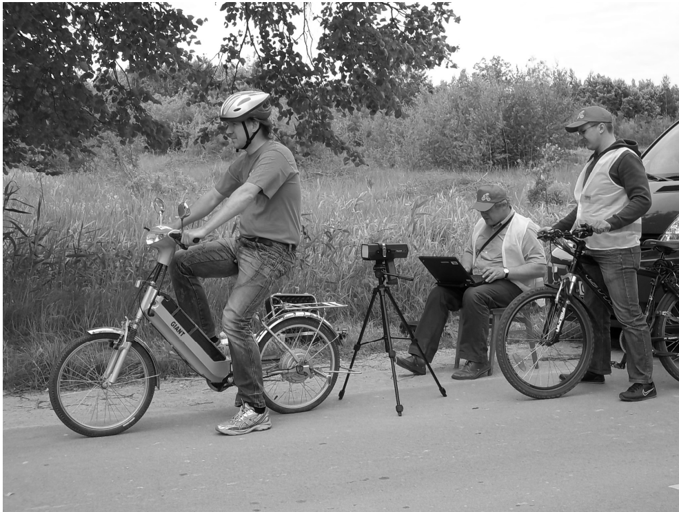
Fig. 2. Electric bicycle acceleration measurement using scientific radar Stalker ATS
